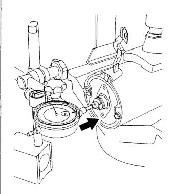
Checking and adjusting armature axial clearance
